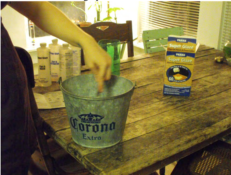
Figure 20: Resin stirred in first container
