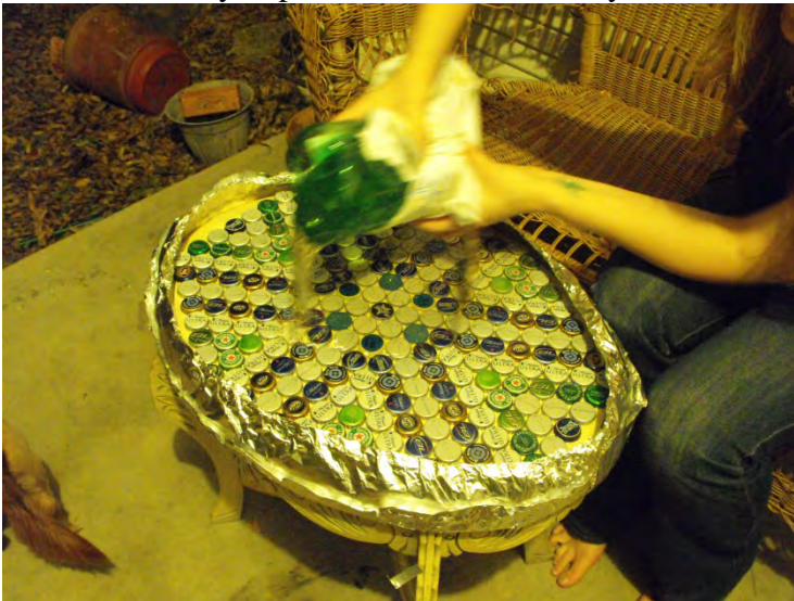
Figure 22: Pouring the resin on the table
