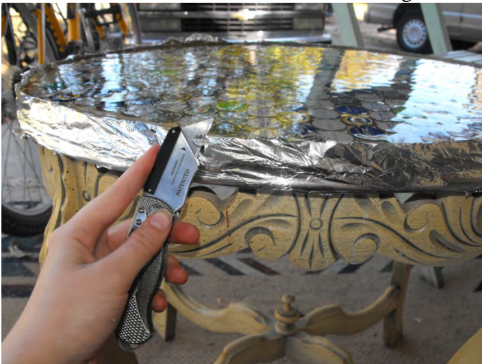
Figure 26: Cutting the resin lip off the table
